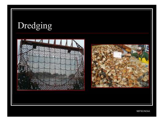
**Dredge** – a heavy metal frame and mesh dragged along the seafloor usually to harvest shellfish (e.g., clams, scallops, cockles). The catch is held in a terminal bag that allows water, sand and mud to wash out, leaving shellfish behind. Bycatch is highly variable with the fishery and dredges can be highly damaging to benthic habitats.
